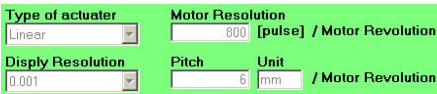
Encoder resolution units and axis mechanical data are read from the connected axis, so the area shown above is used for display only.
