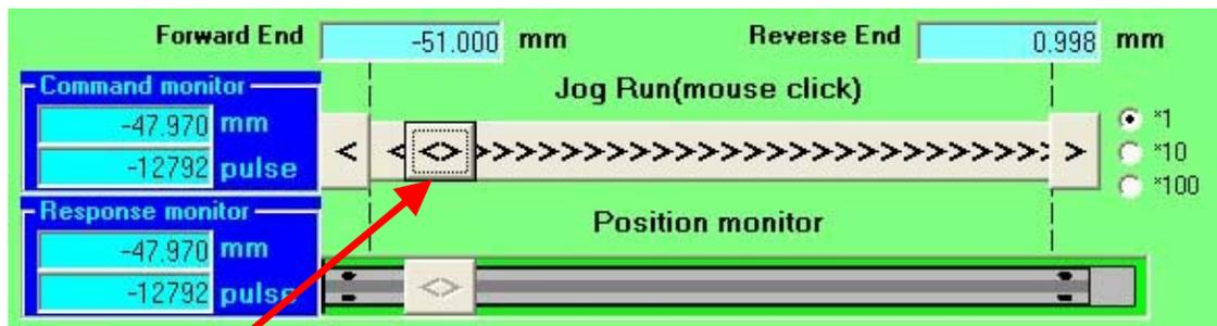
Drag the handle of the jog bar and move it to about [-45mm]; the actuator shaft will move. When the actuator shaft is in the desired position, click the “Position Data Save Window” button to go to the [Position Data Edit Menu].
