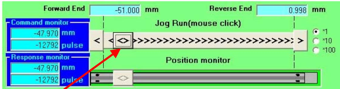
Drag the handle of the jog bar and move it to about [-5mm]; the actuator shaft will move. When the actuator shaft is in the desired position, click the “Position Data Save Window” button to go to the [Position Data Edit Menu].
